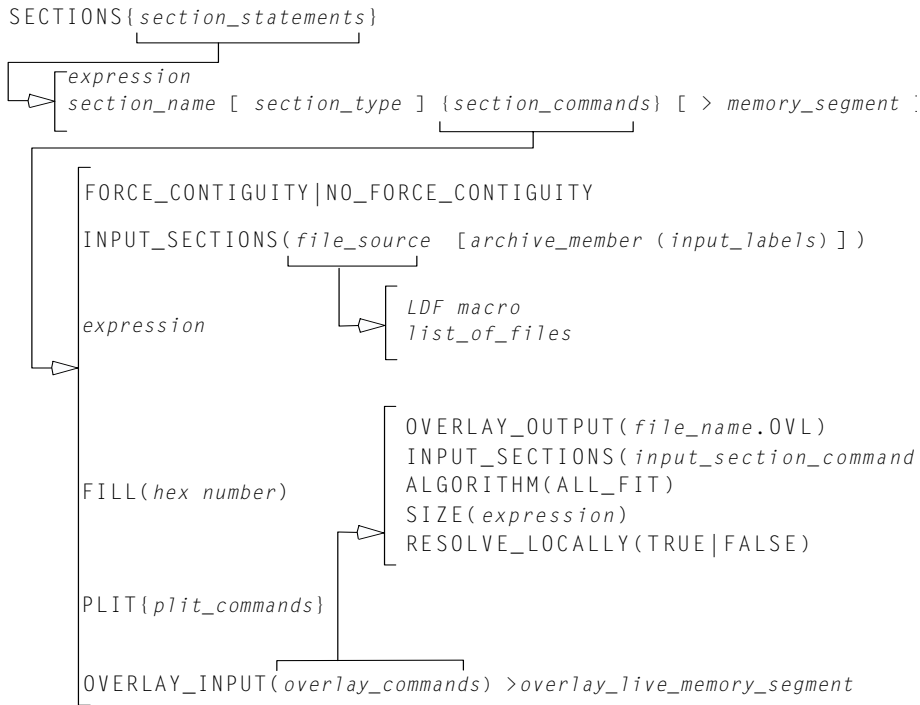
Figure 3-4. SECTIONS{} Command Syntax Tree
