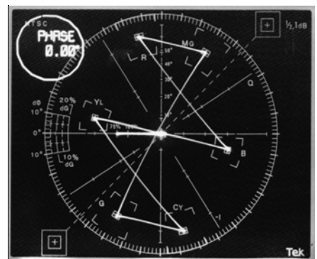
Figure 2.3.4 Vectorscope representation of vector and chroma amplitude relationships in the NTSC system for a color bars signal. (Courtesy of Tektronix.)
