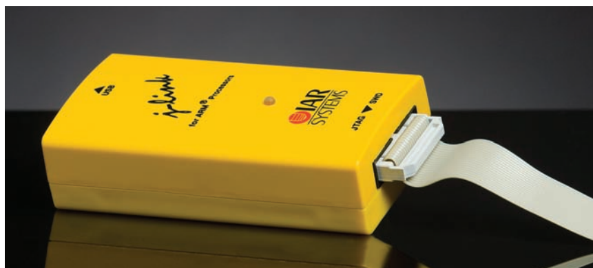
Figure 6 The J-Link debug probe from IAR Systems® can be used to non-intrusively measure both board-level and chip-level power consumption as well as synchronize power sampling with the MCU program counter.
