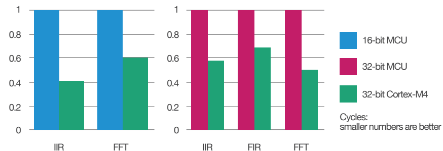
Figure 2 Compared to the leading 16- and 32-bit MCUs with DSP extensions, the STM32 F4’s Cortex-M4 core is twice as efficient when performing the fundamental operations—FIR, IIR, and FFT—that make up a significant portion of communications, audio, and motor control processing.
