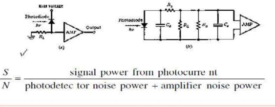
$$\frac{S}{N} = \frac{\left\langle i_P^2 \right\rangle M^2}{2q(I_P + I_D)BM^2 F(M) + 2qI_LB + 4k_BTB/R_L}$$
