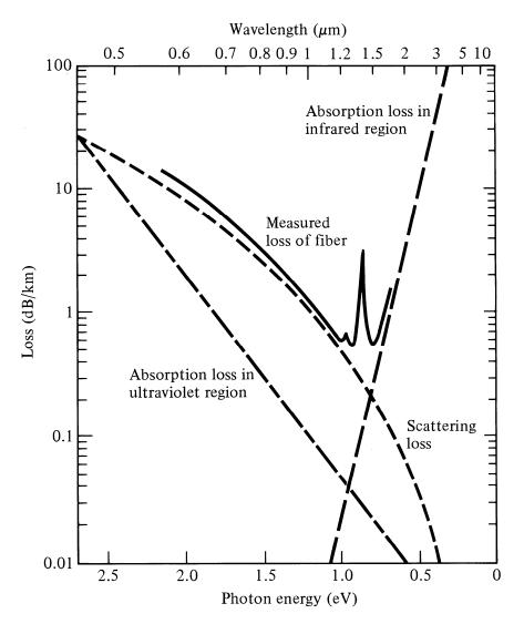
It is interesting to see that in the presence of various losses, there is a natural window in the optical spectrum where the loss is as low as 0.2-0.3dB/Km. This window is from 1200nm to 1600nm.
