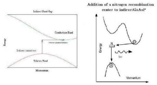
Figure 3: Indirect Bandgap and NonRadiative recombination
