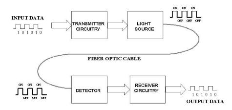
The Receiver circuit consists of a photo detector along with an appropriate electronic circuit, which is capable of measuring magnitude, frequency and phase of the optic field. This type of communication uses the wave lengths near to the <u>infrared band</u> that are just above the visible range. Both LED and Laser can be used as light sources based on the application.
