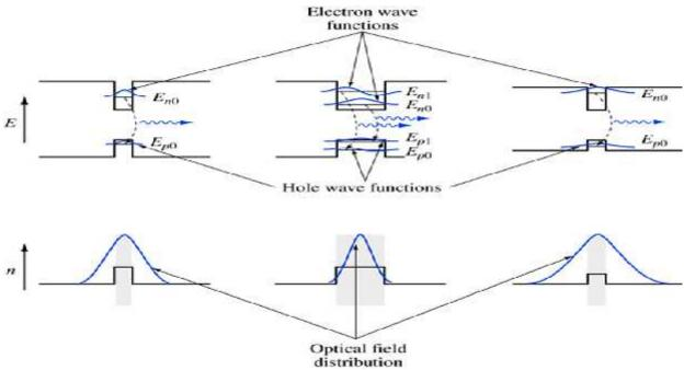
Adjusting the depth and width of quantum wells to select the wavelength of emission is one form of band-gap engineering. The shaded areas indicate the width of the well to illustrate the degree of confinement of the mode.
