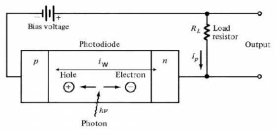
The high electric field present in the depletion region causes photogenerated carriers to separate and be collected across the reverse – biased junction. This gives rise to a current flow in an external circuit, known as **photocurrent**.
