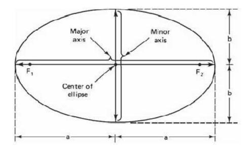
Fig.2.1 The foci *F1* and *F2*, the semimajor axis *a*, and the semiminor axis *b* of an ellips The foci *F* The eccentricity and the semimajor axis are two of the orbital parameters specified for satellites (spacecraft) orbiting the earth. For an elliptical orbit, 0 < e < 1. When e = 0, the orbit becomes circular.
