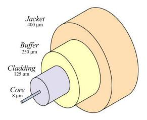
A Fiber Optic Cable consists of four parts.
