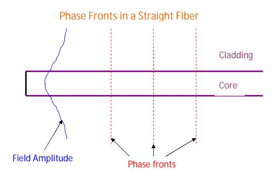
It can be noted that for the straight the phase fronts are parallel and each point on the phase front travels with the same phase velocity.
