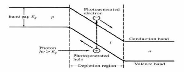
An incident photon is able to boost an electron to the conduction band only if it has an energy that is greater than or equal to the bandgap energy
