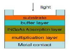
InGaAs APD superlattice structure (The multiplication region is composed of several layers of InAlGaAs quantum wells separated by InAlAs barrier layers.
