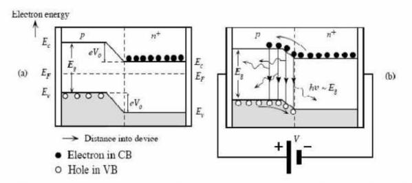
(a) The energy band diagram of a  $pn^+$  (heavily *n*-type doped) junction without any bias. Built-in potential  $V_o$  prevents electrons from diffusing from  $n^+$  to p side. (b) The applied bias reduces  $V_o$  and thereby allows electrons to diffuse or be injected into the *p*-side. Recombination around the junction and within the diffusion length of the electrons in the *p*-side leads to photon emission.
