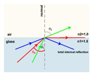
When a light ray crosses an interface into a medium with a higher refractive index, it bends towards the normal. Conversely, light traveling cross an interface from a higher refractive index medium to a lower refractive index medium will bend away from the normal.
