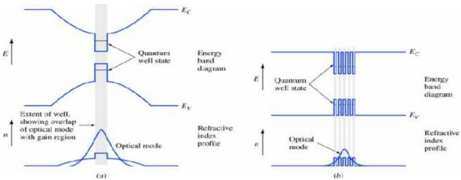
(a) A GRINSCH structure helps funnel the carriers into the wells to improve the probability of recombination. Additionally, the graded refractive index helps confine the optical mode in the nearwell region. Requires very precise control over layers due to grading. Almost always implemented via MBE
