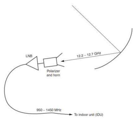
Fig. 4.2 Block schematic for the outdoor unit (ODU)
