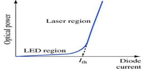
The power-current curve of a laser diode. Below threshold, the diode is an LED. Above threshold, the population is inverted and the light output increases rapidly.
